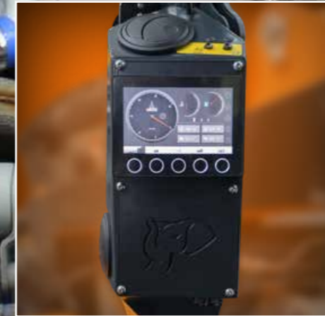
COMPUTER DI BORDO PER CONTROLLO MOTORE DEUTZ ON-BOARD COMPUTER FOR DEUTZ DIESEL ENGINE CONTROL
