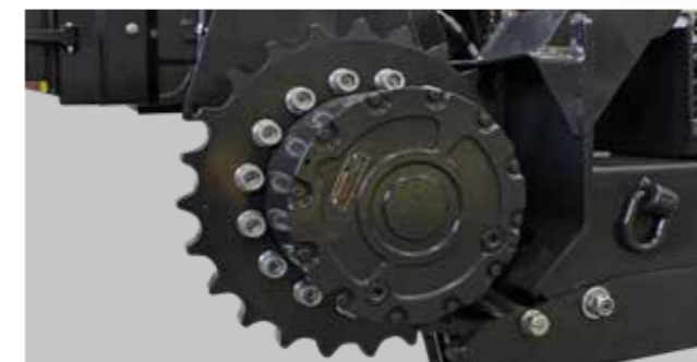
Ruota dentata cingolo in acciaio temperato Gear wheel of transmission to the tracks in hardened steel
